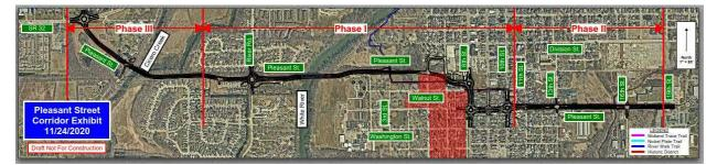
The purpose of the project is to provide significant volume reduction of S.R. 32 downtown Noblesville traffic, defined as 20% reduction. This will meet the project need by addressing the limited mobility in the City of Noblesville by connecting S.R. 32 to S.R. 37 via improvements and new alignment along Pleasant Street. This will provide an alternate method of east-west travel with the City, improving mobility downtown. The following describes the existing and future conditions:
